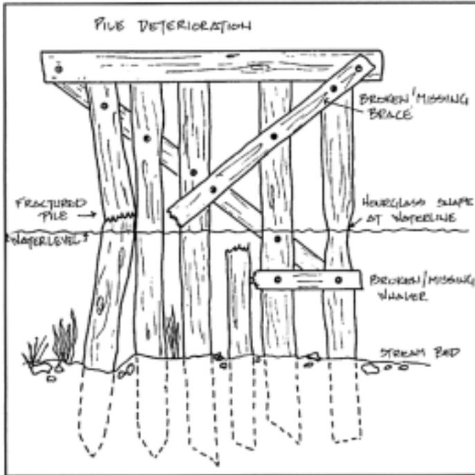
Many rail bridges are supported on timber pile foundations and these should be checked for rot by taking core samples where possible. Some piles may be worn by the endless flow of water, ice and debris. Look for hourglass shape piles at the waterline. Cross bracing make piles act together as a group and is very important. Many of the bridges have loose, broken, or missing braces, and these should be noted, and included in future repairs.
