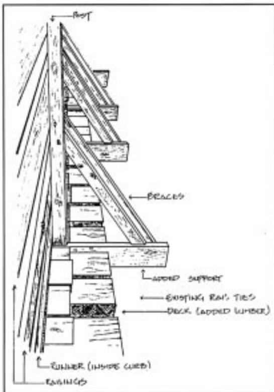
Many of the higher railway bridges have high approaches that may be tens of feet above surrounding grades providing a hazardous vertical drop on both sides leading to the bridge. It is important that the railing system extends past the bridge to protect users from biking or riding off the abutments and possible injury.
